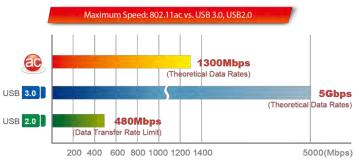
\*USB 3.0 is up to 10 times faster than USB 2.0 and specifies a maximum transmission speed of up to 5Gbps
